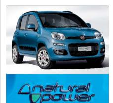
year in the new Fiat Panda (pictured above), combining the environmental benefits of a methane fuel supply with the power and performance of Fiat's Turbo TwinAir technology. It delivers 59 kW at 5500 RPM and 140 Nm of torgue at a low 2500 RPM, whilst consuming just 3.1 kg of methane for every 100 km driven on a combined cycle.
